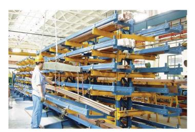
Cantilever Racks are being used for storing tubular products, structure products, section aluminum and many products with long and big sizes. Materials are stored and fixed on the arms by the side forklifts or stacker cranes. This type is suitable for the warehouses with limited space and low height and widely being used in mechanical industries and supermarket of building materials.
