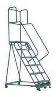
Durable steel ladders are made using 2" x 1" rectangular tubular steel framing. Weight actuated lockstep keeps ladder in position when in use. Safety ladders feature a large 21"D top platform step and 59° slope. 24"W steps are available in 3 styles. Moves easily on non-marring wheels. Rear wheels include corner bumpers to prevent scratching of hallways during transport. Scratch resistant powder coat finish.
